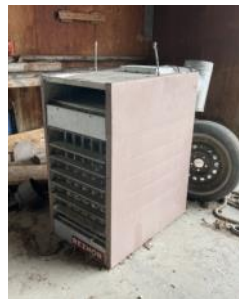
OVERHEAD HEATER (not installed)
